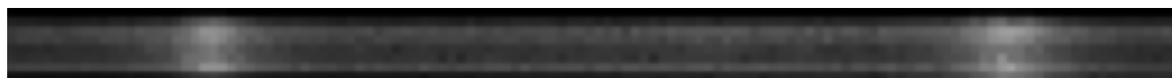
Figure S20. Raw spectral image of the LI mode discharge generated with the Marx generator. This spectral image is 8 pixels height and 1024 pixels wide and was recorded at 2.1 Mfps. The diffraction grating used has 1855 lines per mm and a spectral resolution of 0.38 nm.
