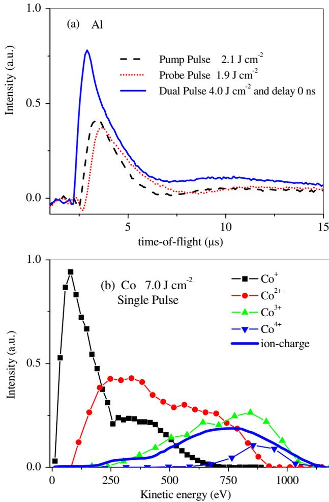
**Figure 2.** (a) T.o.f. signal in the ion collector in DP (solid blue line) and SP experiments (dashed black and short-dotted red lines) with aluminum as target; (b) example of KEDs measured in a SP experiment at  $7.0 \text{ J cm}^{-2}$  of laser fluence and cobalt as target, the ion-charge trace from the ion collector is also shown (see the text).
