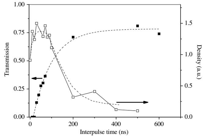
**Figure 7.** Joint plot of the temporal evolution of density and transmission through a laser-produced plasma of aluminum. Data were extracted from DP experiments shown in figures 4 and 5. Lines are guides to the eye.
