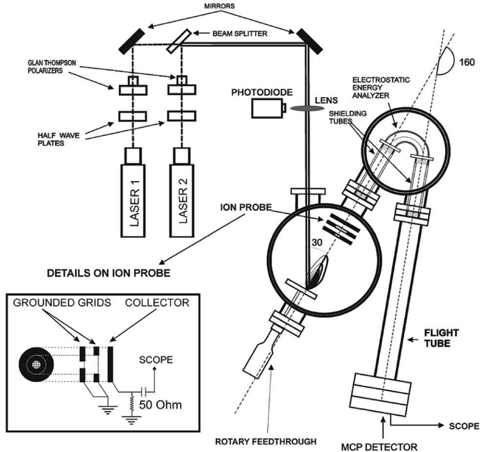
**Figure 1.** Experimental set-up. The ion probe and EEA used in this work are sketched. Details on the ion probe are also shown. The ion collector can be retracted to allow ions fly freely towards the EEA after passing through grounded grids (see text).
