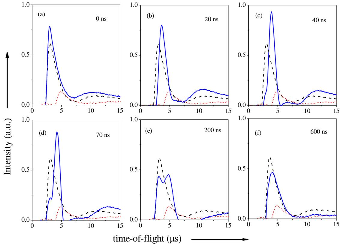
**Figure 5.** Similar to figure 4 but energies of the first and second laser were  $1.0$  and  $3.5 \text{ J cm}^{-2}$ , respectively. Signals at interpulse times of  $0 \text{ ns}$  (a),  $20 \text{ ns}$  (b),  $40 \text{ ns}$  (c),  $70 \text{ ns}$  (d),  $200 \text{ ns}$  (e) and  $600 \text{ ns}$  (f) are shown. The target was aluminum.
