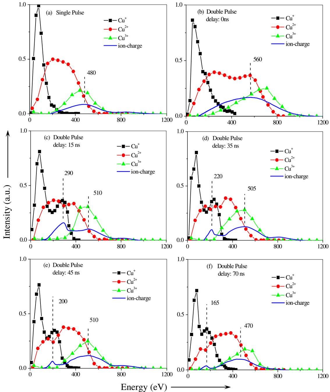
**Figure 6.** Joint representation of KEDs and t.o.f. traces from the transmission grid (solid blue lines) of ions produced in experiments on copper targets. Laser energies used for plasma production and for probing it were both equal to  $1.5 \text{ J cm}^{-2}$ . Results in SP mode (a) and in DP mode at interpulse times of 0 ns (b), 15 ns (c), 35 ns (d), 45 ns (e) and 70 ns (e) are shown.
