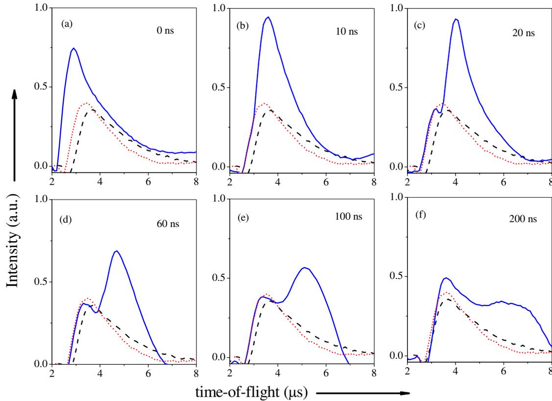
**Figure 3.** T.o.f. traces collected from the ion probe in DP experiments (solid blue lines) at interpulse times of 0 ns (a), 10 ns (b), 20 ns (c), 60 ns (d), 100 ns (e) and 200 ns (e). Laser energies for the plasma and probe lasers were  $2.0 \text{ J cm}^{-2}$  approximately. Dashed black and short-dotted red lines correspond to t.o.f. signals produced for both lasers in SP experiments at these fluences. The target was aluminum.
