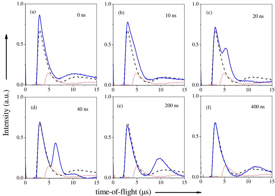
**Figure 4.** T.o.f. traces collected from the ion probe in DP experiments (solid blue lines) at delays of 0 ns (a), 10 ns (b), 20 ns (c), 40 ns (d), 200 ns (e) and 400 ns (f). Laser energies used to produce the plasma and to probe it were  $3.5 \text{ J cm}^{-2}$  and  $1.0 \text{ J cm}^{-2}$ , respectively. Dashed black and short-dotted red lines correspond to t.o.f. signals produced in SP experiments at fluences of  $3.5$  and  $1.0 \text{ J cm}^{-2}$ , respectively. The target was aluminum.
